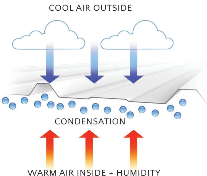
Condensation can be a serious problem in buildings and roof systems. The formation and dripping of condensate can cause damage to building contents, insulation and other components. Using Condenstop enhanced roof panels is an effective and cost efficient solution to help prevent these adverse effects of condensation.
