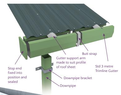
We fabricate a range of gutters including butt straps, stop ends, gutter support arms, outlets and rainwater pipes to customers' requirements. Here are a few examples:
